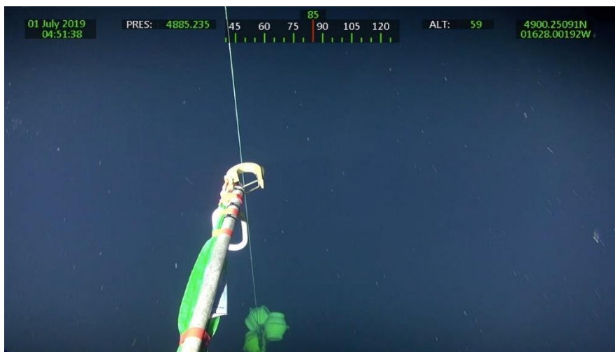
Photo showing glass floats on Bathysnap mooring.
